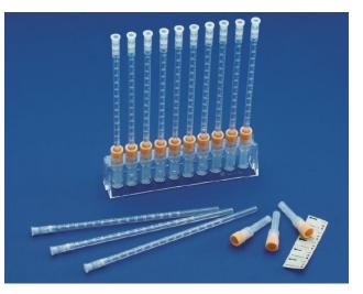
Overall length Graduated scale Bore size Uniformity of bore 200 mm 0-150 ± 0,35 mm 2,5, ± 0,15 mm ±0,05 mm
